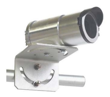
The 18549 mounting bracket uses u-bolts to connect the bracket to a crossarm. Curved notches allow the camera to be aimed at the desired target.
