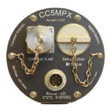
The connectors on the back of the CC5MPX have metal caps that are chained to the camera.
