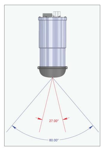
The CC5MPX has a 4 to 12 mm lens, which provides an approximate 27° horizontal field of view when fully zoomed in and an 80° horizontal field of view when fully zoomed out.
